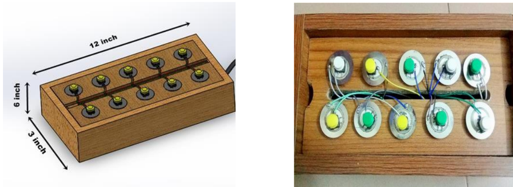
Fig. 4. Schematic view of prototype wooden keyboard.
